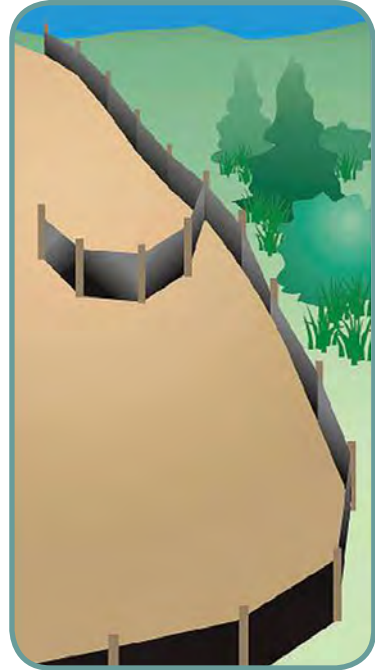
Use J-hooks to trap and pond muddy runoff flowing along the uphill side of the silt fence. Turn ends of the silt fence toward the uphill side to prevent bypassing.
