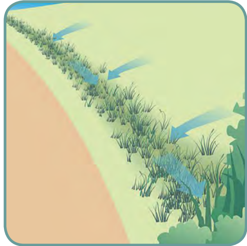
Diversion channels should be stabilized
